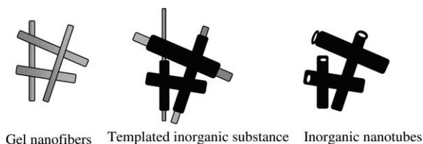
**Fig. 19** Schematic representation of templated synthesis of metal oxide nanotubes.
