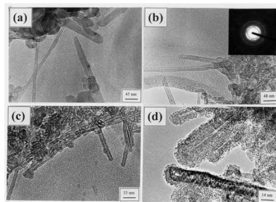
**Fig. 20** TEM images of the titania nanotubes (a) as-synthesized and (b)–(d) after calcination. Inset shows the SAED pattern taken on a single nanotube. Reproduced with permission from ref. 77a ©2003 The Royal Society of Chemistry.
